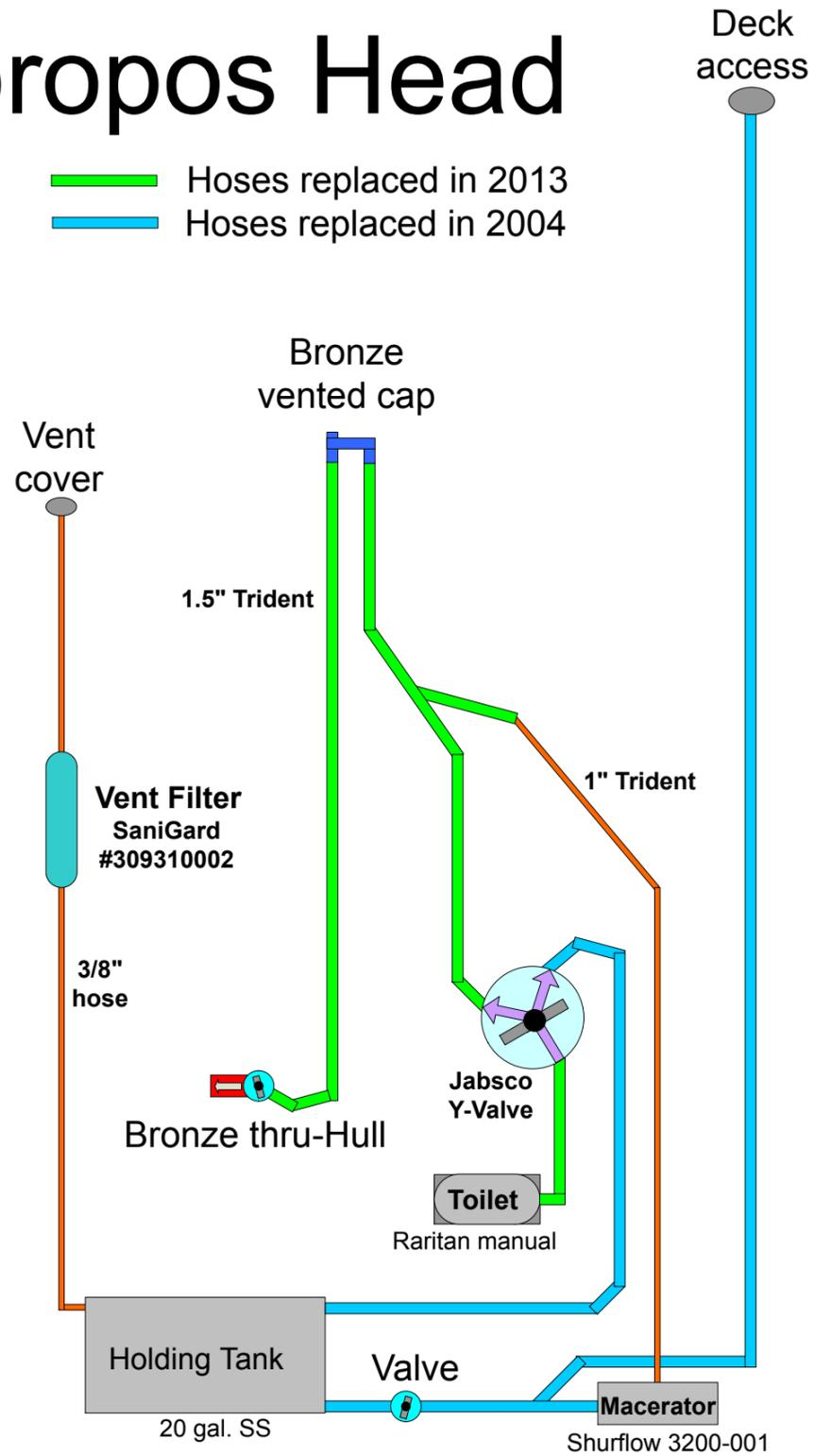
**Note:** 1" hose from macerator to Y connector needs to be flushed periodically using macerator after filling deck access hose with fresh water with holding tank valve closed.
